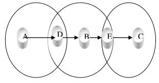
Fig.2 Communication between node A and C via intermediate node D, B, E
